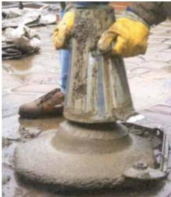
Initial Mix with 1.5 in slump, before addition of AERFLOW™
