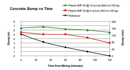
Reference Mix used a Type A Water Reducer Dosage of 4 oz/100 lbs (260 mL/100 kg cement)
